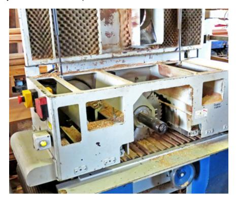
The saw blades are mounted on a common arbor with a mechanical arrangement which allows the distance between the blades to be adjusted up to 24 inches.
