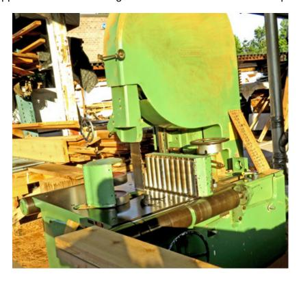
Standing over 6 feet tall and equipped with an estimated 4" wide blade and a massive power feeder, this machine looked more than capable of handling the milling of any chunk of wood that could be hoisted onto the table!
